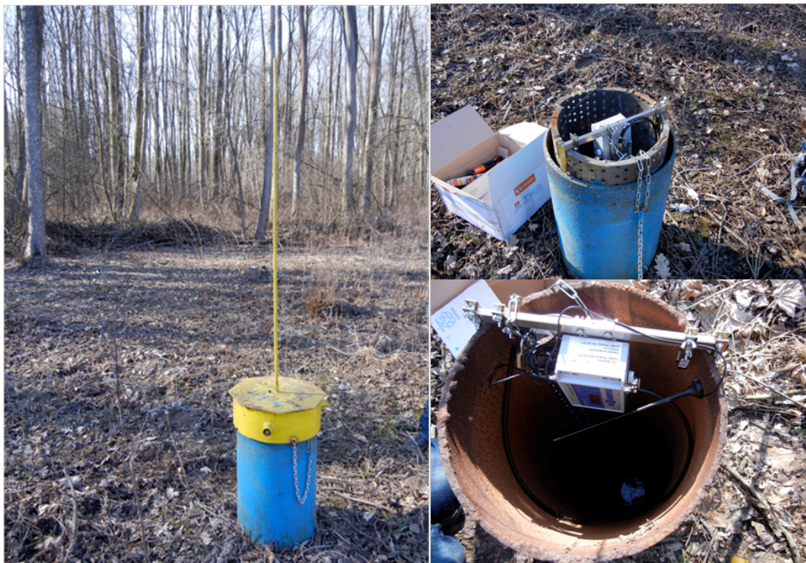
Figure 7 Installation of pressure sensor for single drill
