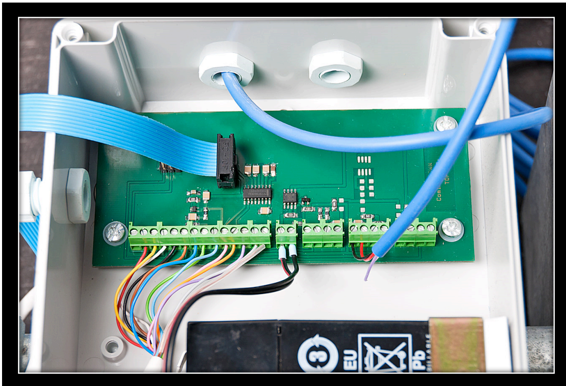
Figure 9 Prototype PCB - sensor inputs, control of sensor power management of each sensor
