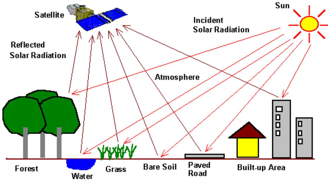
Figure 3 Physics of reflectance; energy source, transmission path, target and the satellite sensor
