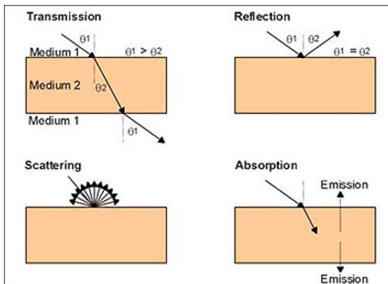
**Figure 5** Any beam of photons from some source passing through medium 1 (usually air) that impinges upon an object or target (medium 2) ([http://rst.gsfc.nasa.gov/Intro/Part2\\_3.html](http://rst.gsfc.nasa.gov/Intro/Part2_3.html))
