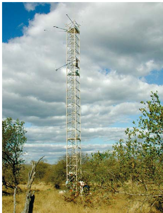
Flux tower for in-situ carbon-dioxide measurements
